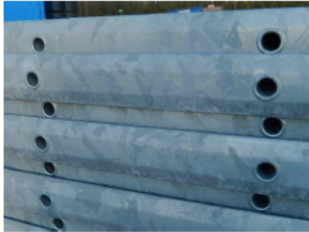
Image 2, Ladders matured with a healthy oxide layer
