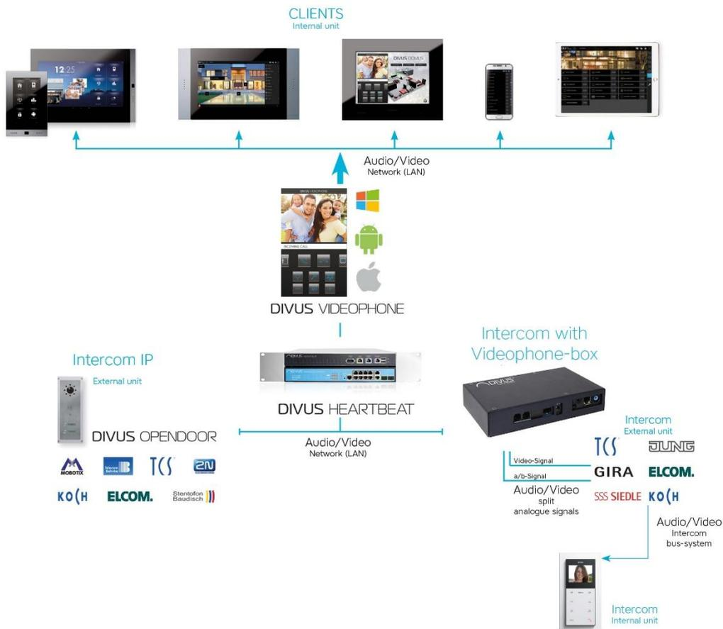
For most common cases, the DIVUS HEARTBEAT may be used as a plug and play VoIP server, meaning that just setting the clients' configurations using our default configuration scheme will cause them to just connect and work – without any intervention on the DIVUS HEARTBEAT's configuration itself.
