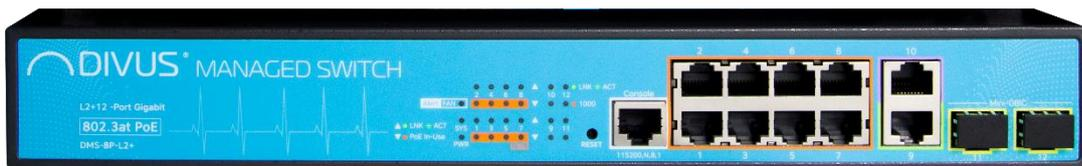
The MANAGED SWITCH is an 8 ports full PoE+ switch, with two additional ports to connect to other devices in a chain. It is known to the manager, which is therefore able to not only talk directly to the devices attached to the switch, but also to log and show all the switch's activities in great detail. Any number of DMS may be attached to the main DMS using its dedicated ports 9 and 10 (*cascading*).
