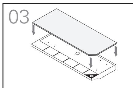
Apply the adhesive supplied to the plastic base. If this adhesive is not used, there may be problems with incorrect fastening.
