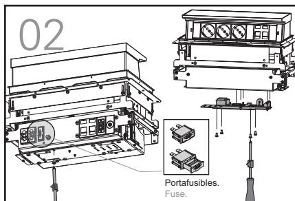
Loosen the lower protective cover and unscrew the card access cover as shown in figure 2. Disconnect the cables and replace with new ones; connect the cables and screw on the card access, replace the lower protective cover.
