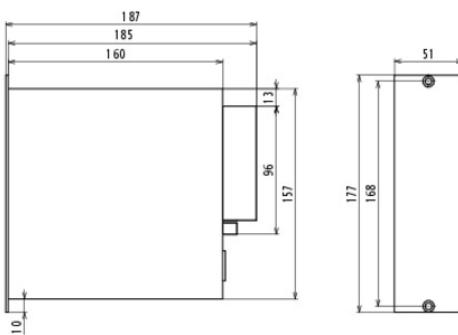
DSRT DD FS .... detection device for light detection (DSRT FS fibre optic sensor).
